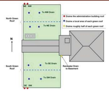
Figure 2. There are two green roof test systems, one on the North Bay, and one on the South Bay. Each of the green roofs has two drainage areas dividing the roof approximately in half. The Office Roof System has gutters that catch runoff from the south and east sides and drains to holding tanks in the basement.
